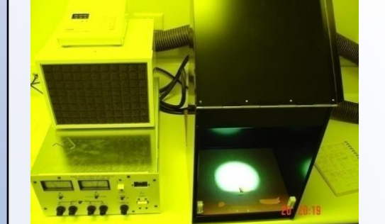
Figure 6. OAI deep UV illumination system (Model LS30/5) fitted with a 500W HgXe-lamp for the surface modification and in situ preparation of the organic polymer monolith in the polypropylene pipette tips, and photografting of reactive vinylazlactone group for trypsin immobilization.
